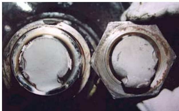
(b) Straight view at the two broken faces
