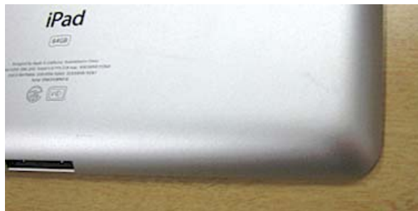
Fig. 7 iPad has continuous curvature on its edge
